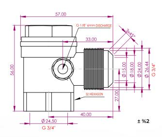
MAY-40 Compressor Check Valve is designed using CNC machines with first-grade MS58 brass (according to EN12164 standards), ensuring high airflow capacity and 30 bar operating pressure. Thanks to its specially designed impact-resistant gasket, it is durable up to +250°C without oil absorption. Developed by YKS engineers, MAY Series Compressor Check Valves provide a reliable solution for industrial compressors.
