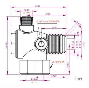
MAY-20/F Compressor Check Valve is designed using CNC machines with first-grade MS58 brass (according to EN12164 standards), ensuring high airflow capacity and 30 bar operating pressure. Thanks to its specially designed impact-resistant gasket, it is durable up to +250°C without oil absorption. Developed by YKS engineers, MAY Series Compressor Check Valves provide a reliable solution for industrial compressors.
