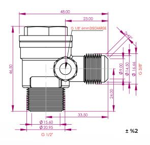
MAY-35 Compressor Check Valve is designed using CNC machines with first-grade MS58 brass (according to EN12164 standards), ensuring high airflow capacity and 30 bar operating pressure. Thanks to its specially designed impact-resistant gasket, it is durable up to +250°C without oil absorption. Developed by YKS engineers, MAY Series Compressor Check Valves provide a reliable solution for industrial compressors.
