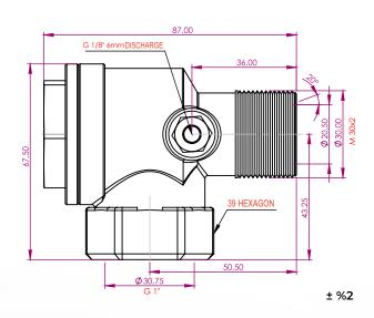
MAY-30/2D Compressor Check Valve is designed using CNC machines with first-grade MS58 brass (according to EN12164 standards), ensuring high airflow capacity and 30 bar operating pressure. Thanks to its specially designed impact-resistant gasket, it is durable up to +250°C without oil absorption. Developed by YKS engineers, MAY Series Compressor Check Valves provide a reliable solution for industrial compressors.
