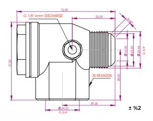
MAY-25/F Compressor Check Valve is designed using CNC machines with first-grade MS58 brass (according to EN12164 standards), ensuring high airflow capacity and 30 bar operating pressure. Thanks to its specially designed impact-resistant gasket, it is durable up to +250°C without oil absorption. Developed by YKS engineers, MAY Series Compressor Check Valves provide a reliable solution for industrial compressors.
