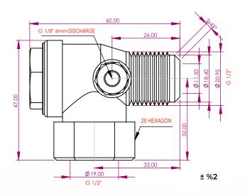
MAY-15/F Compressor Check Valve is designed using CNC machines with first-grade MS58 brass (according to EN12164 standards), ensuring high airflow capacity and 30 bar operating pressure. Thanks to its specially designed impact-resistant gasket, it is durable up to +250°C without oil absorption. Developed by YKS engineers, MAY Series Compressor Check Valves provide a reliable solution for industrial compressors.
