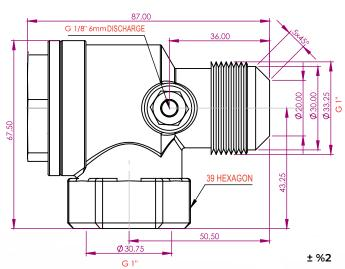
MAY-30 Compressor Check Valve is designed using CNC machines with first-grade MS58 brass (according to EN12164 standards), ensuring high airflow capacity and 30 bar operating pressure. Thanks to its specially designed impact-resistant gasket, it is durable up to +250°C without oil absorption. Developed by YKS engineers, MAY Series Compressor Check Valves provide a reliable solution for industrial compressors.
