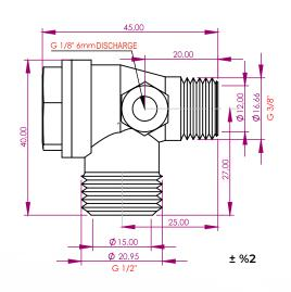
MAY-5 Compressor Check Valve is designed using CNC machines with first-grade MS58 brass (according to EN12164 standards), ensuring high airflow capacity and 30 bar operating pressure. Thanks to its specially designed impact-resistant gasket, it is durable up to +250°C without oil absorption. Developed by YKS engineers, MAY Series Compressor Check Valves provide a reliable solution for industrial compressors.
