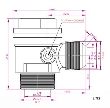
MAY-45 Compressor Check Valve is designed using CNC machines with first-grade MS58 brass (according to EN12164 standards), ensuring high airflow capacity and 30 bar operating pressure. Thanks to its specially designed impact-resistant gasket, it is durable up to +250°C without oil absorption. Developed by YKS engineers, MAY Series Compressor Check Valves provide a reliable solution for industrial compressors.
