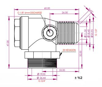
MAY-15 Compressor Check Valve is designed using CNC machines with first-grade MS58 brass (according to EN12164 standards), ensuring high airflow capacity and 30 bar operating pressure. Thanks to its specially designed impact-resistant gasket, it is durable up to +250°C without oil absorption. Developed by YKS engineers, MAY Series Compressor Check Valves provide a reliable solution for industrial compressors.
