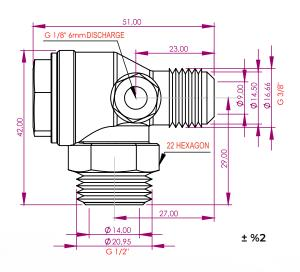
MAY-10 Compressor Check Valve is designed using CNC machines with first-grade MS58 brass (according to EN12164 standards), ensuring high airflow capacity and 30 bar operating pressure. Thanks to its specially designed impact-resistant gasket, it is durable up to +250°C without oil absorption. Developed by YKS engineers, MAY Series Compressor Check Valves provide a reliable solution for industrial compressors.
