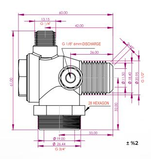
MAY-20 Compressor Check Valve is designed using CNC machines with first-grade MS58 brass (according to EN12164 standards), ensuring high airflow capacity and 30 bar operating pressure. Thanks to its specially designed impact-resistant gasket, it is durable up to +250°C without oil absorption. Developed by YKS engineers, MAY Series Compressor Check Valves provide a reliable solution for industrial compressors.
