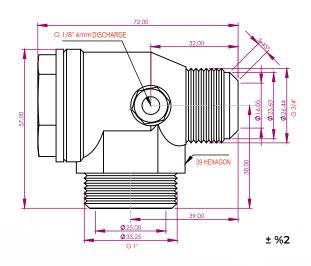
MAY-25 Compressor Check Valve is designed using CNC machines with first-grade MS58 brass (according to EN12164 standards), ensuring high airflow capacity and 30 bar operating pressure. Thanks to its specially designed impact-resistant gasket, it is durable up to +250°C without oil absorption. Developed by YKS engineers, MAY Series Compressor Check Valves provide a reliable solution for industrial compressors.
